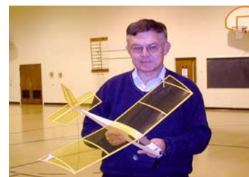
Woody flies in small gyms with the Hitec Feather receiver, 7 cell 50 mah flight pack, or 3 CR2 Lithiums and 2 HS 55 servos.
