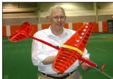
Firefly ROG for Motors up to Speed 280 size, 48-inch wingspan, NACA 6409 Undercambered airfoil
